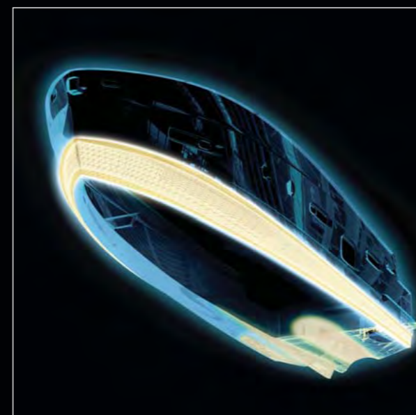
Dual Mode semi-planing hull with tunnel, skag and vertical bow (Magellano Collection)
