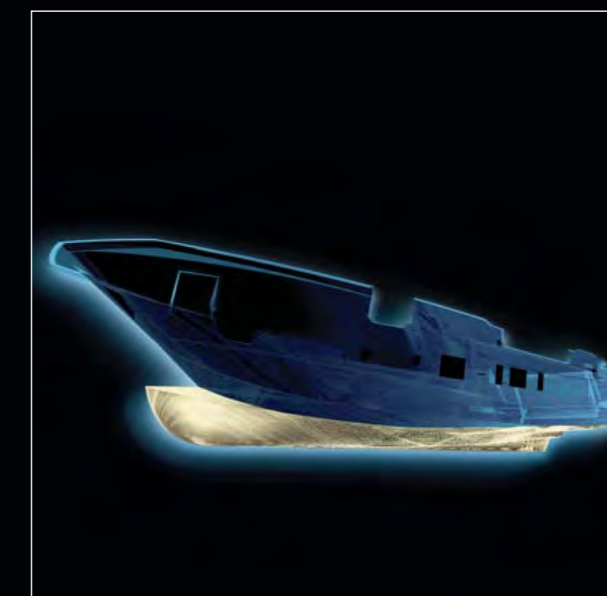
D2P (Displacement to Planing) hull with a double chine and wave piercer (reserved for several models in the Grande Collection)
