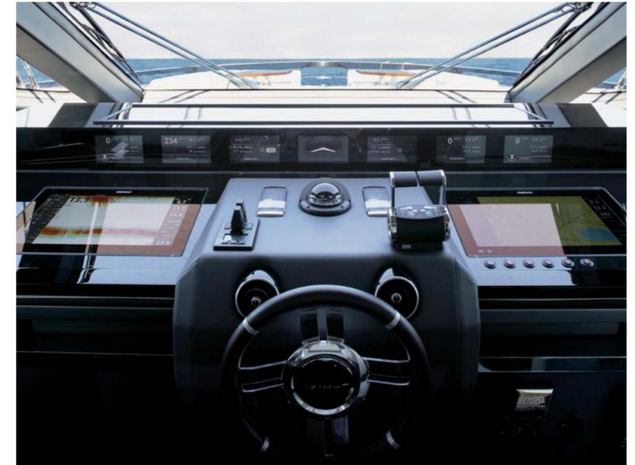
*The bridge was produced in partnership with Simrad-Naviop and has a single ultra-wide screen displaying key monitoring and navigation information, a mix of video sources and clusters of content. Accessing this information is easy with a choice of commanders or two touch screens duplicated by a pair of physical jockers for extra redundancy and safety.*
