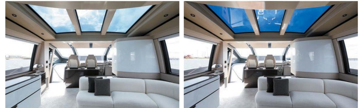
*The saloon's ceiling features an electrochromic glass skylight, a laminated panel incorporating an electro-optical film based on SPD (Suspended Particles Device) technology. This system, which is based on an electrical field that aligns the particles in the film, filters light and UV rays so as to provide greater comfort and wellbeing.*
